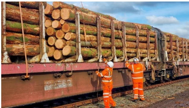
Figure 3 Railway ground staff preparing the strapping of a timber train prior to departure.
