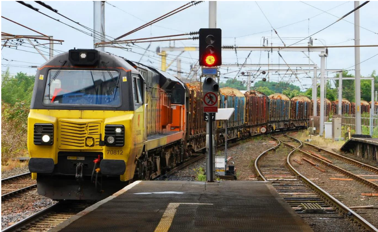
Figure 5 Example of a Colas Rail hauled timber service for Kronospan utilising 'KFA'/'IWA' type wagons.
